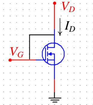
Fig. 4 NMOS Diode Connected Configuration.
