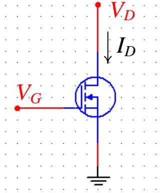
Fig. 3 NMOS I-V Measurement Configuration.
