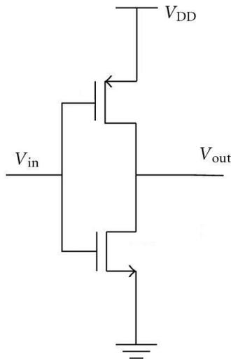
**Figure 4:** CMOS Inverter Circuit
