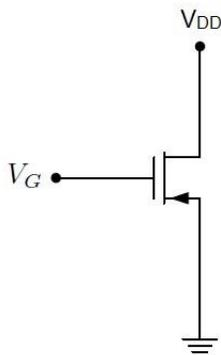
Figure 2: PMOS I-V Measurement Configuration
