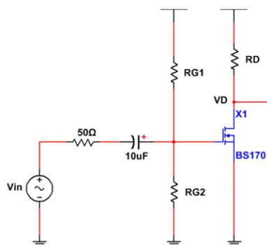
**Figure 2:** First stage circuit topology.
