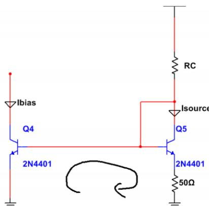
**Figure 5:** Current source circuit
