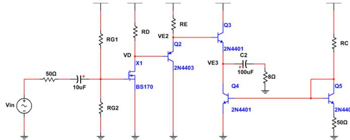
**Figure 1:** Circuit topology for Lab 5.
