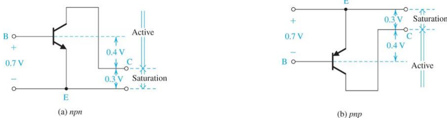
Figure 4.14 Graphical representation of the conditions for operating the BJT in the active mode and in the saturation mode.
