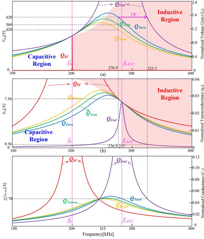
Fig. 8. Dc voltage and current characteristics of the LCC charger.
