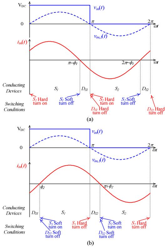
Fig. 3. Switching output waveforms in continuous conduction mode for resonant converters with (a) capacitive  $Z_m$ , and (b) inductive  $Z_m$ .
