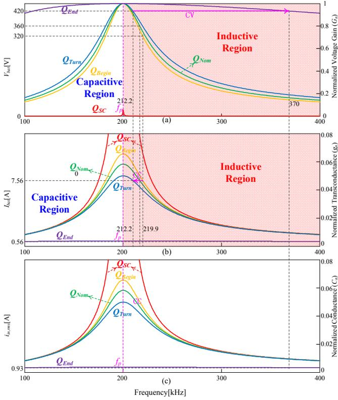
Fig. 6. Dc voltage and current characteristics of the SRC charger.
