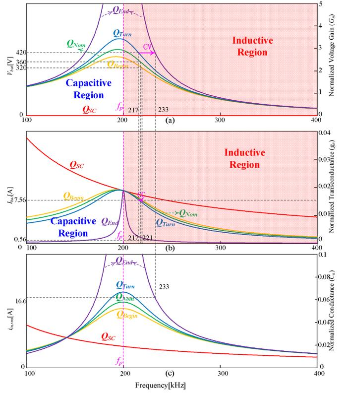
Fig. 7. Dc voltage and current characteristics of the PRC charger.
