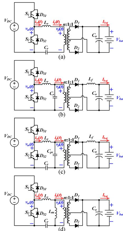
Fig. 1. Isolated resonant topologies in battery charging applications. (a) Series resonant converter (SRC). (b) Parallel resonant converter (PRC). (c) LCC series-parallel resonant converter (LCC). (d) LLC series-parallel resonant converter (LLC).
