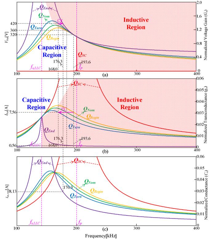
Fig. 9. Dc voltage and current characteristics of the LLC charger.
