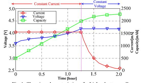
Fig. 4. Charging characteristics of a Li-Ion battery cell.
