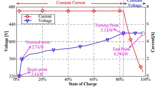
Fig. 5. Charging profile of a 360 V Li-Ion battery pack rated at 3.2 kW.
