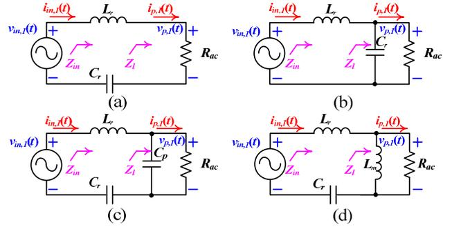
Fig. 2. Ac equivalent models of resonant converters. (a) SRC. (b) PRC. (c) LCC. (d) LLC.
