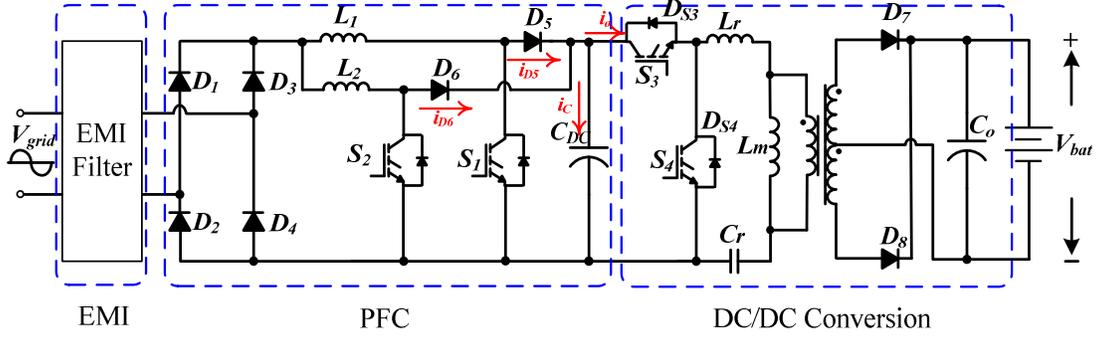
Fig. 2. Schematic of proposed interleaved level 2 isolated on board charger.
