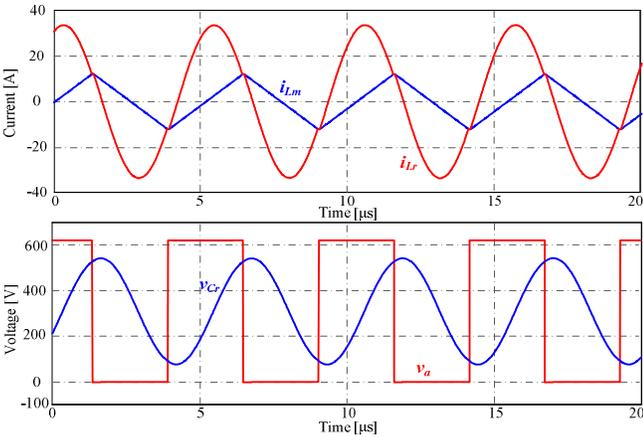
Fig. 14. LLC results at the begin point ( $V_o = 320$  V,  $I_o = 19.1$  A,  $f = 195$  kHz).
