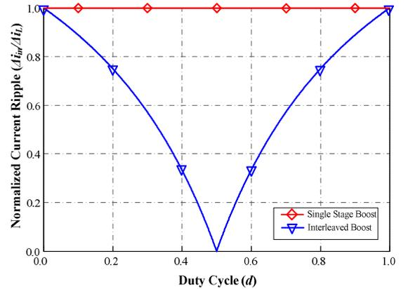
Fig. 4. Effective input current ripple cancellation in two-leg interleaved converter.
