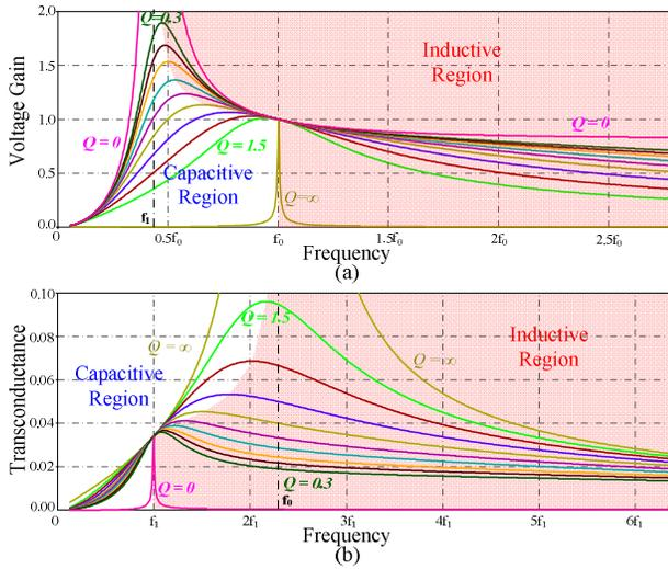
Fig. 8. Dc characteristic of LLC resonant converter: (a) voltage characteristic (b) current characteristic.
