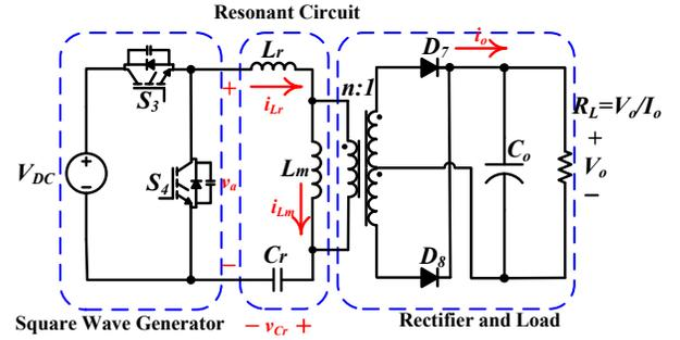
Fig. 6. Schematic of an LLC resonant half-bridge converter.
