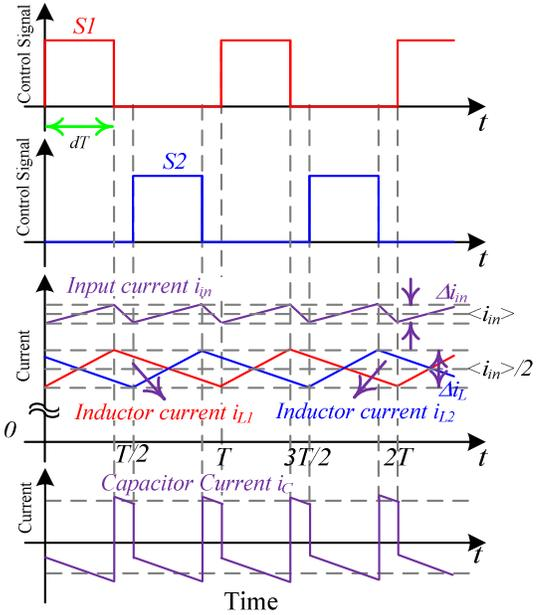
Fig. 3. Waveforms of two-leg interleaved boost converter ( $d < 0.5$ ).
