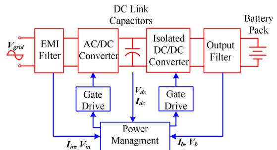
Fig. 1. General system architecture of a battery charger
