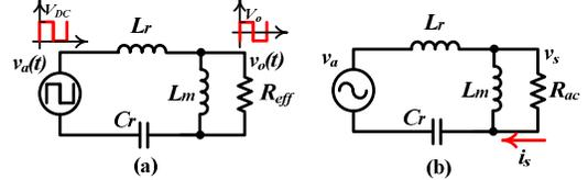
Fig. 7. (a) Simplified LLC half-bridge converter circuit. (b) Circuit model under first harmonic approximation (FHA).
