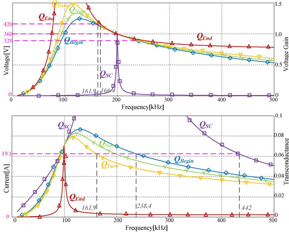
Fig. 12. Dc characteristics of the designed 7.6kW LLC converter: a) voltage characteristic b) current characteristic.
