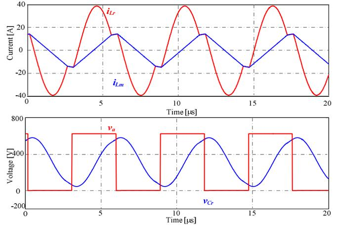
Fig. 15. LLC results at the nominal point ( $V_o = 360$  V,  $I_o = 19.1$  A,  $f = 171$  kHz).
