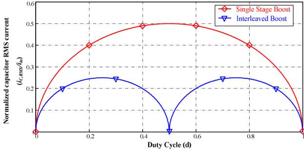
Fig. 5. Effective output capacitor rms current reduction in two-leg interleaved converter.
