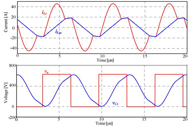
Fig. 16. LLC results at the turning point ( $V_o = 420$  V,  $I_o = 19.1$  A,  $f = 151$  kHz).
