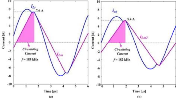
Fig. 12. Performance comparison at the maximum power point (420 V, 2.38A); a) conventional LLC topology; b) proposed hybrid topology.
