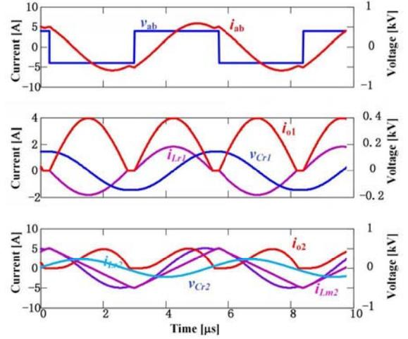
Fig. 14. Simulation waveforms at  $P = 856$  W,  $V_o = 360$  V.
