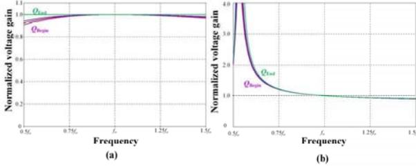
Fig. 13. Comparison of dc voltage gain characteristics in PEV battery charging application; a) conventional SRC topology; b) proposed hybrid topology.
