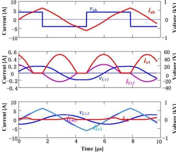
Fig. 17. Simulation waveforms at  $P = 100 \text{ W}$ ,  $V_o = 420 \text{ V}$ .
