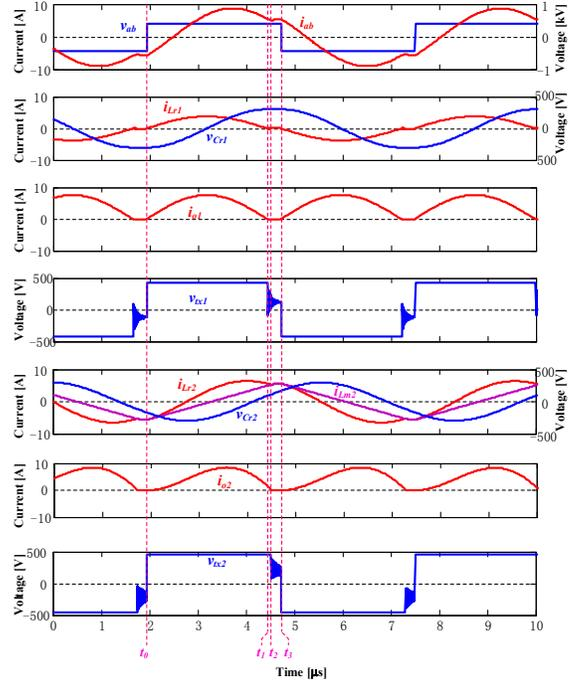
Fig. 11. Key waveforms of the proposed hybrid converter.
