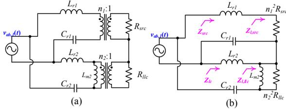
Fig. 9. Circuit model of proposed hybrid converter under FHA.
