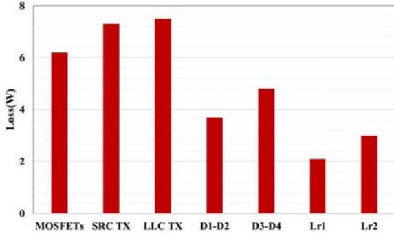
Fig. 18. Loss estimation at 1 kW operation.
