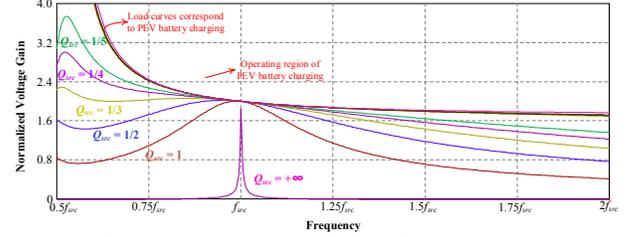
Fig. 8. Dc gain characteristics of proposed hybrid converter under different load variations.
