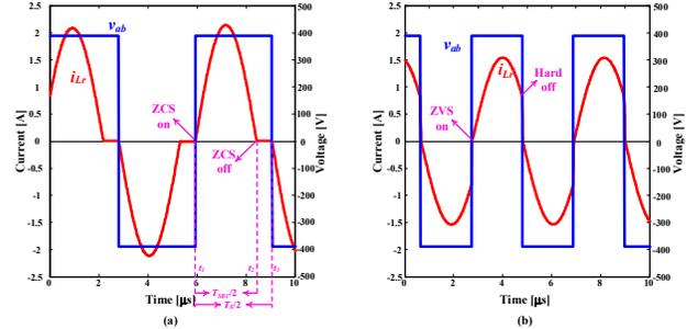
Fig. 4. Operation comparison of SRC converter in a) region 1; and b) region 2.
