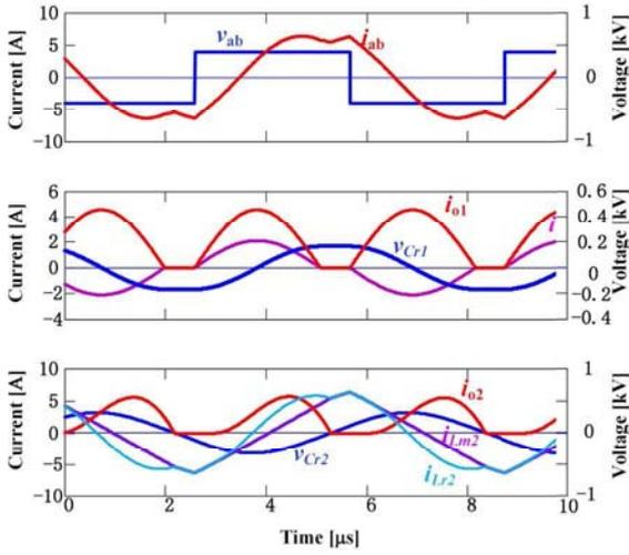
Fig. 16. Simulation waveforms at  $P = 1 \text{ kW}$ ,  $V_o = 420 \text{ V}$ .
