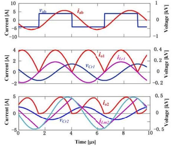
Fig. 15. Simulation waveforms at  $P = 928$  W,  $V_o = 390$  V.
