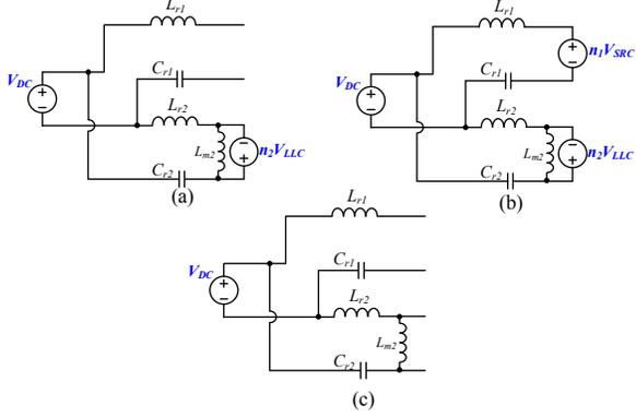
Fig. 10. Equivalent circuits during one half switching cycle; (a) mode 1; (b) mode 2; (c) mode 3.
