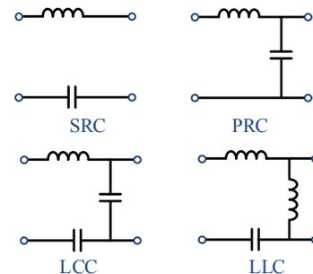
Fig. 2. Four most common typical resonant tank networks.
