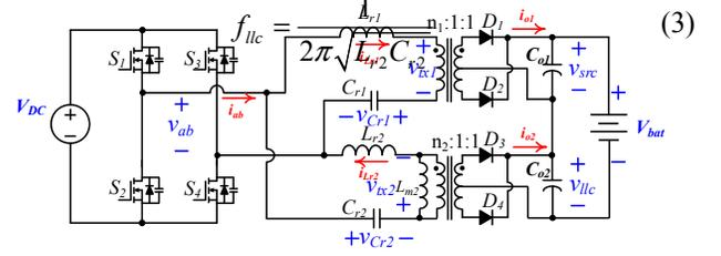
Fig. 7. Proposed hybrid SRC, LLC resonant dc/dc converter.
