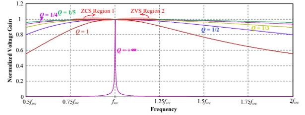
Fig. 3. Dc gain characteristics of SRC converter under different load variations.
