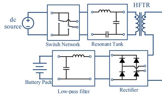
Fig. 1. Block diagram of a conventional resonant dc/dc converter.
