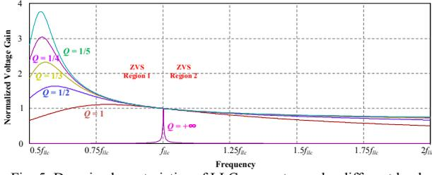
Fig. 5. Dc gain characteristics of LLC converter under different load variations.
