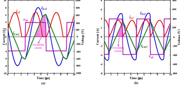
Fig. 6. Operation comparison of LLC converter in a) region 1; and b) region 2.
