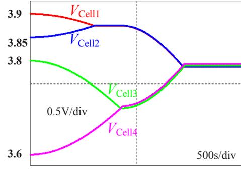
Fig. 7. Simulated balancing process of four series- connected capacitors.
