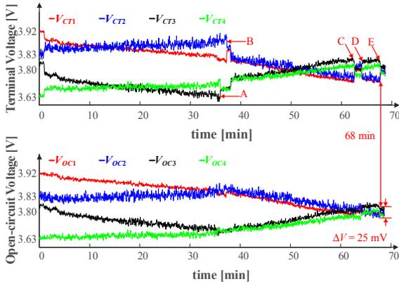
Fig. 11 The open circuit voltage ( $V_{OC}$ ) and terminal voltage ( $V_{CT}$ ) of the four cells
