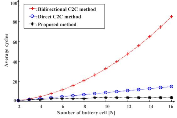
Fig. 6 The average cycles for charge transfer of each method.
