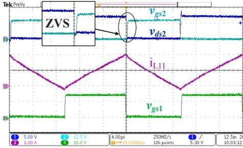
Fig. 10  $v_{gs2}$ ,  $v_{ds2}$  of  $S_{w2}$ ,  $v_{gs1}$  of  $S_{w1}$  and the inductor current  $i_{L1}$ .
