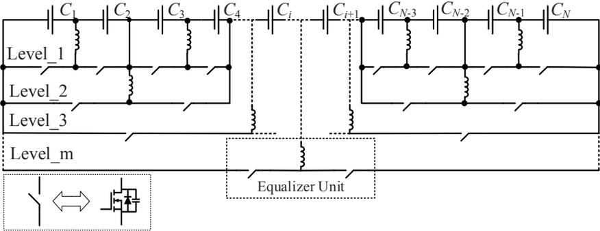
Fig. 1 The hierarchical equalizer schematic based on buck-boost converter.
