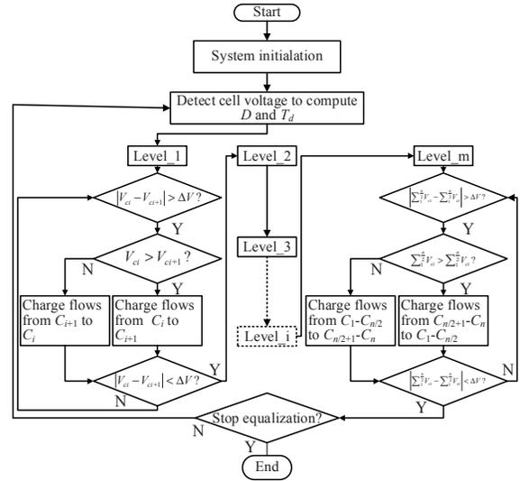
Fig. 5 The control flowchart of the equalizer.
