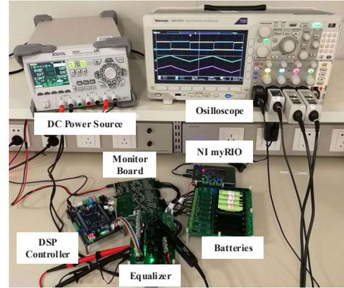
Fig. 8 The photo of experiment setup.
