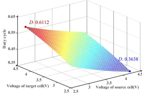
Fig. 4 The variation scope of duty cycle.
