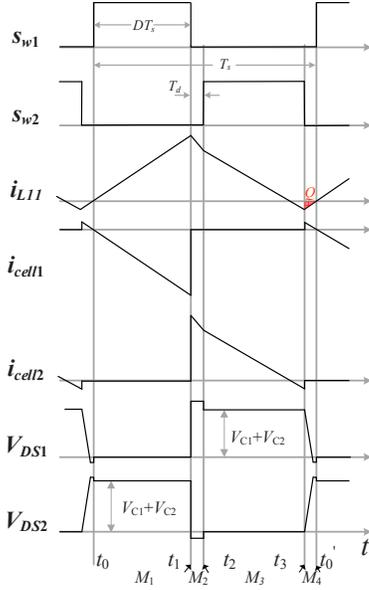
Fig. 2 The key waveforms of the basic equalization unit.
