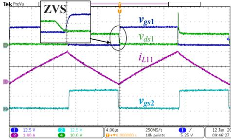
Fig. 9  $v_{gs1}$ ,  $v_{ds1}$  of  $S_{w1}$ ,  $v_{gs2}$  of  $S_{w2}$  and the inductor current  $i_{L1}$ .
