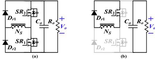
Fig. 21. (a) Modified secondary-side rectifier proposed in [9] (b) Its critical operation mode.
