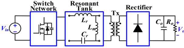
Fig. 1. Block diagram of typical LLC resonant converter.
