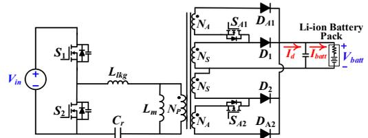
Fig. 10. Reconfigured LLC converter with adaptive turns ratio [17].
