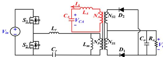
Fig. 7. Modified LLC converter with auxiliary LC circuit [5].
