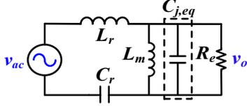
Fig. 2. Ac equivalent circuit model of conventional LLC resonant converter.
