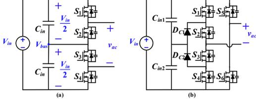
Fig. 14. Topology of modified primary-side inverter. (a) Three-level bridge structure [23]. (b) Three-level full-bridge structure [35].
