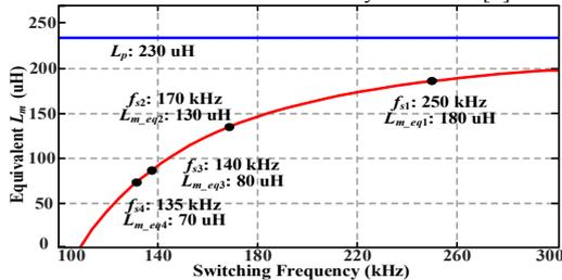
Fig. 8. Equivalent  $L_m$  varies with switching frequency [2].
