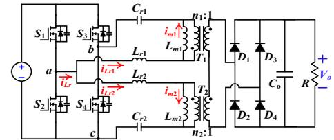
Fig. 12. Modified LLC converter with two split resonant tank [38].
