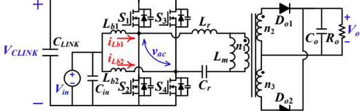
Fig. 16. Interleaved Boost-Integrated LLC (IBI-LLC) converter [42].
