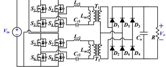
Fig. 18. Topology of interleaved LLC converter [44].
