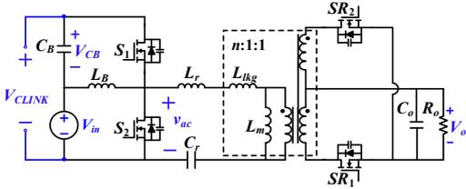
Fig. 15. Buck-boost + LLC cascaded converter [39].
