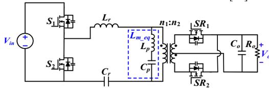
Fig. 6. Topology of LCLC converter [2].
