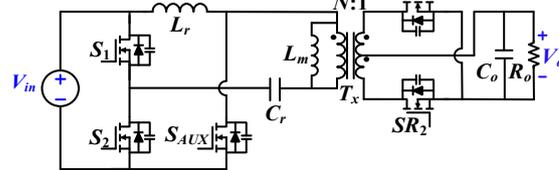
Fig. 19. Modified LLC converter with primary-side auxiliary switch [45].
