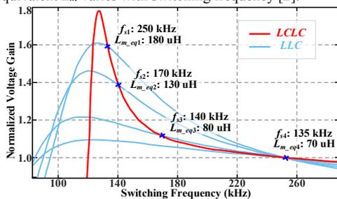
Fig. 9. Gain curves of LCLC and equivalent LLC [2].
