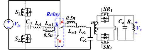
Fig. 11. Reconfigured LLC converter with adaptive turns ratio [37].
