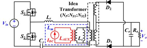
Fig. 5. Modified LLC converter with variable inductance [10].
