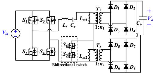
Fig. 4. Two-transformer LLC converter [11].
