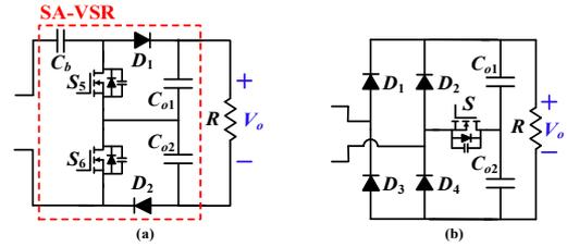
Fig. 20. Topology of modified secondary-side rectifier. (a) SA-VSR structure [52]. (b) Modified voltage doubler structure [31].
