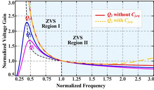
Fig. 3. DC gain curves of conventional LLC resonant converter.
