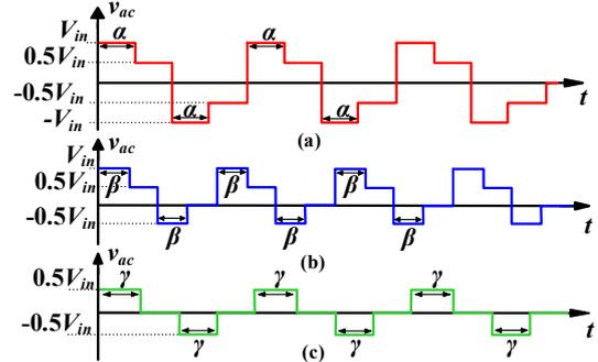
Fig. 17. Waveforms of  $v_{ac}$  proposed in [40]. (a) HG mode. (b) MG mode. (c) LG mode.
