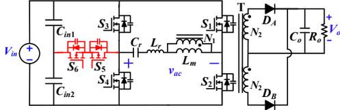
Fig. 13. Dual bridge LLC converter [41].
