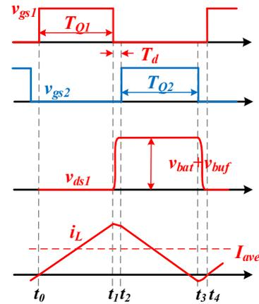
Fig. 3. Key waveforms of bidirectional equalizer unit at BCM operation.
