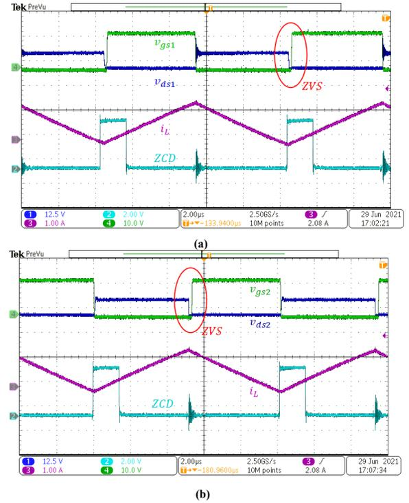
Fig. 11. Key waveforms of steady state  $i_L$ , ZCD signal and MOSFET voltage. (a)  $v_{gs1}$  and  $v_{ds1}$ , (b)  $v_{gs2}$  and  $v_{ds2}$ .
