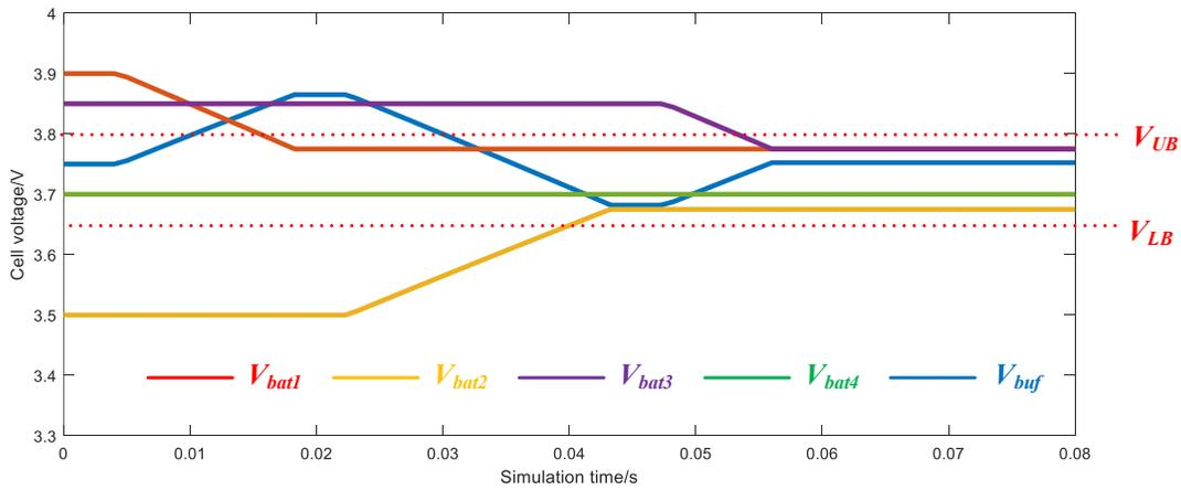
Fig. 12. Simulation result of balancing process.
