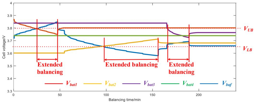
Fig. 13. Measured voltage of batteries and buffer in balancing process with manually zero current detection.
