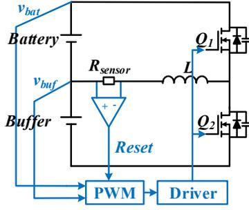
Fig. 6. Zero current detection (ZCD) to realize BCM.
