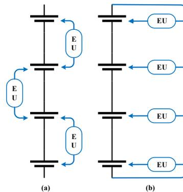
Fig. 1. Typical active equalization topologies (EU: Equalizer unit). (a) Cell-to-Cell equalization, (b) Pack-to-Cell equalization.
