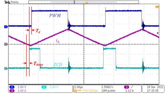
Fig. 10. Key waveforms of ZCD validation.
