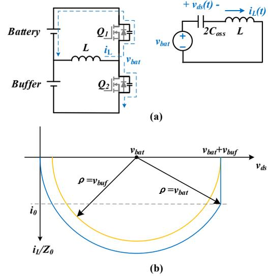
Fig. 5. ZVS analysis. (a) Equivalent circuit of equalizer unit in dead time, (b) Trajectory of ZVS analysis.
