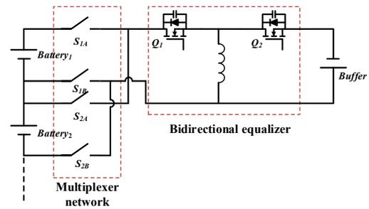
Fig. 2. Schematic of the proposed C2B equalizer
