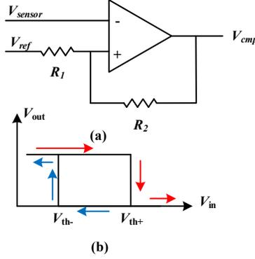
Fig. 7. ZCD method using high-speed comparator. (a) Semantic of ZCD circuit. (b) Hysteresis curve of comparator.
