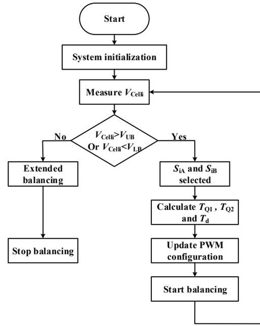
Fig. 8. The flow chart when one cell out of preset operation region is recognized and start balancing.
