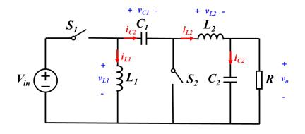
In a period, when  $0 \le t \le DT_s$ , switch  $S_1$  turns on,  $S_2$  turns off; when  $DT_s \le t \le T_s$ , switch  $S_1$  turns off,  $S_2$  turns on.
