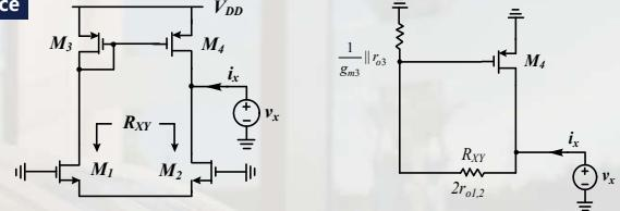
When  $v_x$  is applied to measure  $R_o$ ,  $v_{g4}$  varies!
