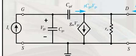
$$I_o = g_m V_{gs} - s C_{gd} V_{gs} = (g_m - s C_{gd}) V_{gs}$$
